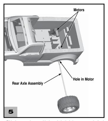
• Slide the rear axle assembly through the hole in one motor, the back end of the vehicle and then out through the other motor.
